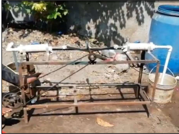
Fig 1: Bicycle operated pedal power water pump
